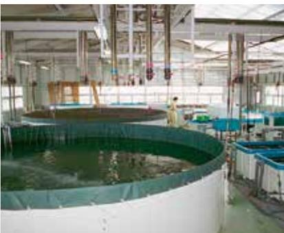
Equipped with outlets for seawater, groundwater and aeration supply to enable various experiments with aquatic organisms.
