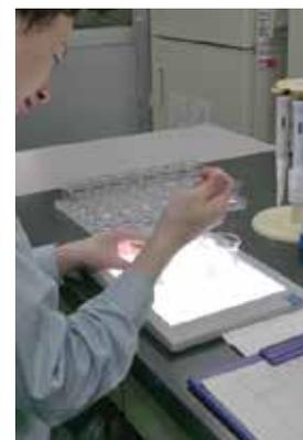
Whole effluent toxicity test (daphnia reproduction test)
