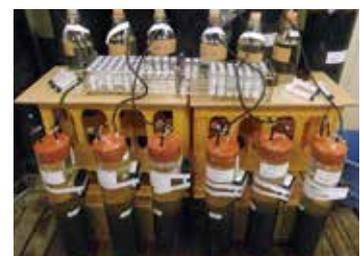
Experiments for estimation of nutrient leaching and denitrification rates
