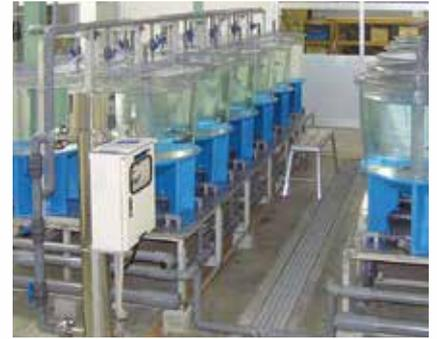
Equipped with closed circulatory culture system for aquatic organisms, thus enabling testing in the isolated condition.
