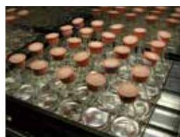
Algal and fish toxicity testing apparatus
