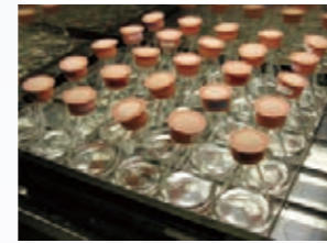
Algae test apparatus (continuous culture)
