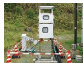
Speciated mercury sampling in the atmosphere
