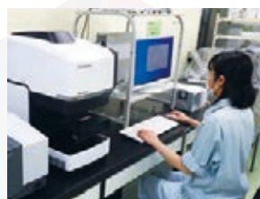
Analysis of MP by FT-IR microscopy
