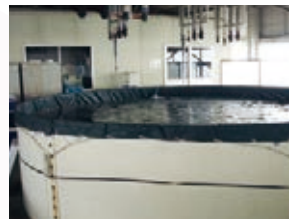
Experimental tank with natural seawater flowing over it
