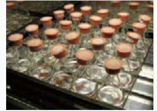
Algae test apparatus (continuous culture)
