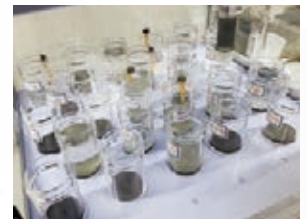
CO 2 absorption test in air and water using steel slag utilization material
