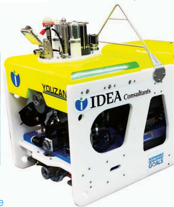
Hovering type AUV, developed in-house: YOUZAN
