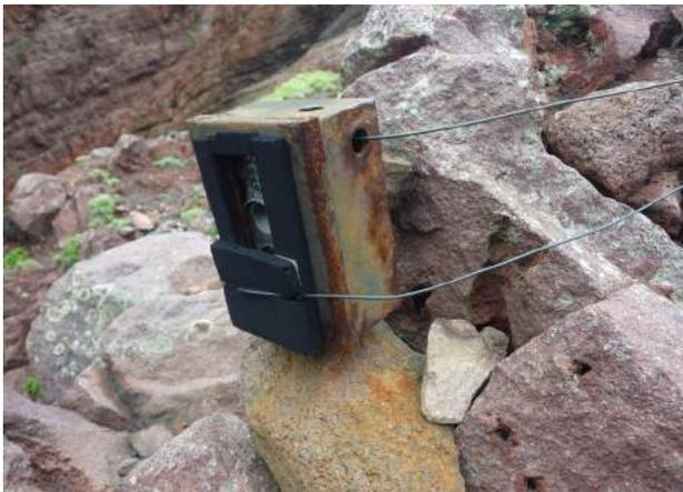
Fig. 2. Time-lapse camera (Ltl Acorn 6210) in metal housing, installed at Tsubamezaki on Torishima
