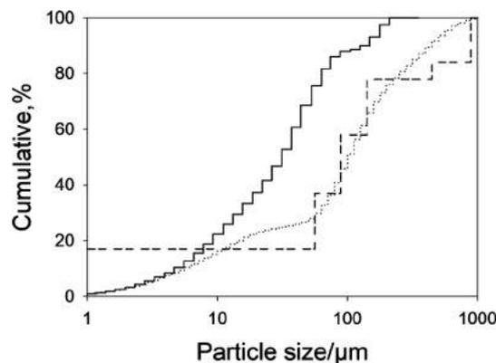
Fig. 2 Cumulative particle size. Broken, dotted, and solid lines indicate the rolling ball mill, roll crusher and pin mill, and combination of roll crusher and pin mill and air jet mill, respectively.
