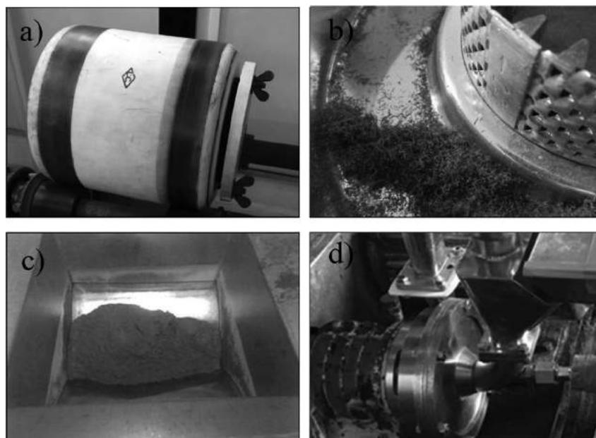
Fig. 1 Grinding apparatuses assessed in this study. a) Rolling ball mill; b) cutting mill; c) roll crusher and pin mill; d) air jet mill.
